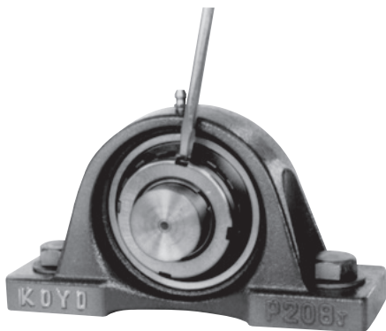
Fig. 14.8 Bending outer tab of washer (Locking locknut)
