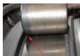
Signs of temperature rise on the roller large end face
