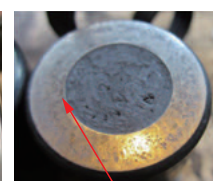
Scuffing occurrence on the roller large end face
