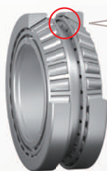
Signs of temperature rise on the roller large end face
