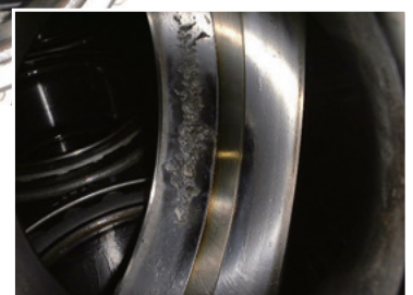
Cracks from the Double-peaked wear on the outer ring, flaking on the raceway surface of outer rings
