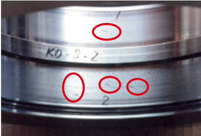
Brinelling on raceway surface of outer ring
