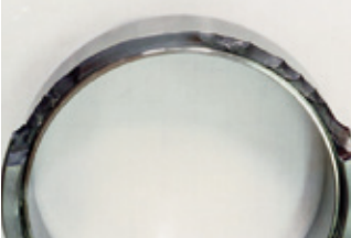
Inner ring cracking
