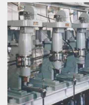
Fig. 3 Rolling fatigue life test conditions and test equipment
