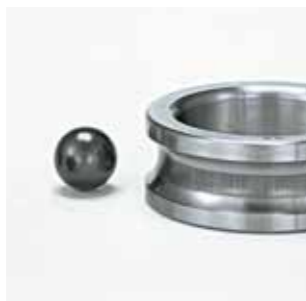
Fig. 18 Electric pitting generated on general purpose bearings (ridges)
