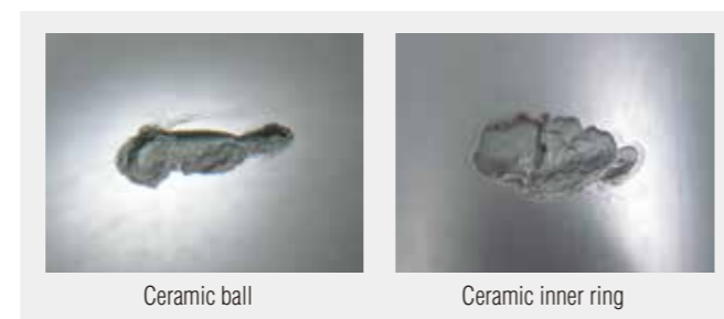
Fig. 6 Flaking on ceramic ball and inner ring
