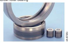
Discoloration on inner ring and roller of Tapered Roller Bearing
