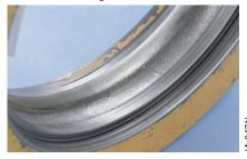
■Brinelling on inner ring raceway surface of Tapered Roller Bearing
