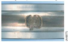
Flaking on inner ring of Cylindrical Roller Bearing
