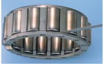
Rust on Tapered Roller bearing cage
