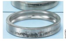
▲ False brinelling on inner ring raceway surface of Deep Groove Ball Bearing
