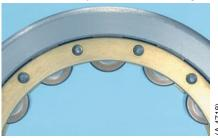
Wear on outer ring raceway surface of Double-Row Cylindrical Roller Bearing
