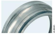
■Smearing on outer ring raceway surface of Cylindrical Roller Bearing
