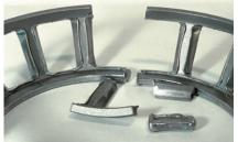
Distortion of Cylindrical Roller Bearing cage
