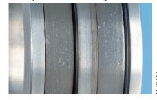
Pear skin on inner ring raceway surface of Deep Groove Ball Bearing
