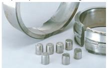
■ Crack on outer ring of Four-Point Contact Ball Bearing
