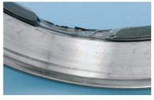
Chip in outer ring rib of Cylindrical Roller Bearing
